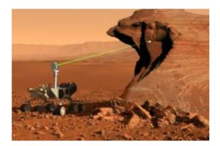
The ChemCam system uses a laser to take samples from as far as 23 feet away from the Curiosity rover.
