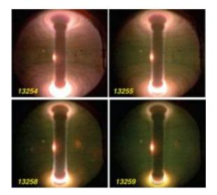
As more lithium is added (with increasing discharge number in yellow), the plasma light changes from red (from recycling of the deuterium fuel gas) to green (lithium emission from the edge of the plasma) and the overall (recycling) light levels decrease. Credit: Princeton Plasma Physics Laboratory
