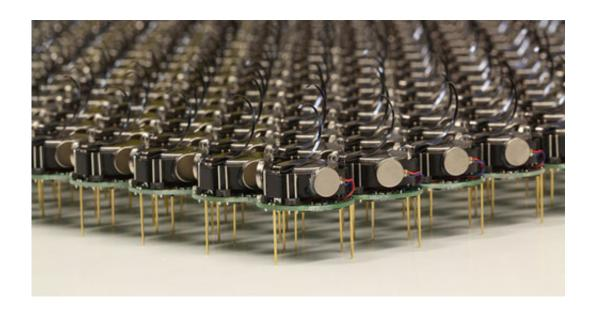
The Kilobots are an inexpensive system for testing synchronized and collaborative behavior in a very large swarm of robots. Photo courtesy of Michael Rubenstein
