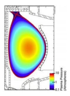
Surfaces of constant plasma pressure in the cross-section of the C-Mod tokamak for an I-mode plasma. In the hottest core region, the pressure exceeds 4 atmospheres. The volume average pressure is over 1.5 atmospheres, more than 50 percent of the central pressure expected in the ITER device, and close to the current tokamak world record of 1.8 atmospheres, also attained on C-Mod Credit: Earl S. Marmar, MIT
