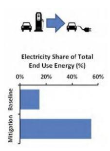
Step 3: Most direct fossil fuel uses in transport, buildings, and industry must switch to electricity, raising the electricity share of end-use energy from 15 percent today to 55 percent in 2050.
