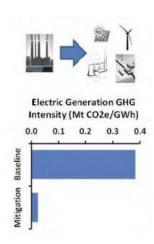
Step 2: Electric generation emissions intensity must be reduced to less than 0.02 kilograms of CO2 emissions per kilowatt-hour.
