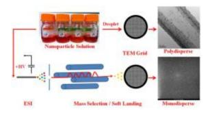
With the soft-landing approach, identical particles are evenly distributed on the sample.
