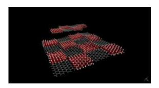
Making a superlattice with patterns of hydrogenated graphene is the first step in making the material suitable for organic chemistry. The process was developed in the Rice University lab of chemist James Tour. Credit: Tour Lab/Rice University
