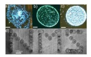
Dark field optical micrograph of inkjet printed drops on a) plasma cleaned, b) pristine and c) HMDS treated substrate. Scale: 20µm. d) SEM micrograph of printed pattern. Image from arXiv:1111.4970v1 [cond-mat.mtrl-sci]
