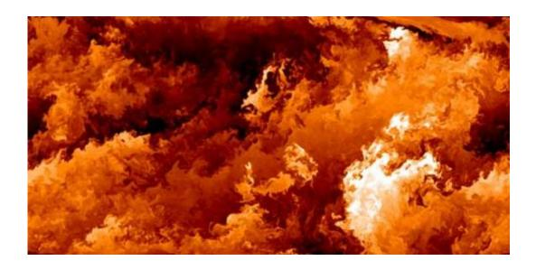
Direct numerical simulation of stratified turbulence. Lighter colors correspond to denser fluid. Image: Georgios Matheou and Daniel Chung
