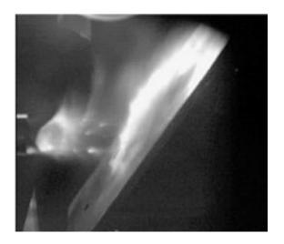
A large (+16 mm) pellet is undergoing testing for ITER disruption mitigation. The pellet, on the left, is exiting the guide tube just before hitting a simple target plate. It will shatter once it hits the plate. (Photo: Combs, ORNL)
