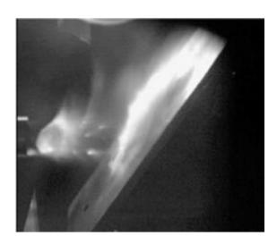
A large (+16 mm) pellet is undergoing testing for ITER disruption mitigation. The pellet, on the left, is exiting the guide tube just before hitting a simple target plate. It will shatter once it hits the plate. (Photo: Combs, ORNL)
