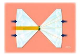
This illustration depicts a diamond anvil cell which allows to compress microscopic pieces of material to pressures of 3 Mbar and more. Laser pulses (black arrows) then heat the sample and an X-ray beam (orange) passes through the cell to probe the states of matter at these extreme conditions. Credit: ESRF/Format Editions
