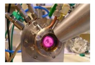
This image shows the heating of a catalyst sample in an "in situ" cell at actual operating conditions. The catalyst is studied using time-resolved X-ray absorption spectroscopy. At ID24, the time resolution can be as short as a few microseconds. Credit: ESRF
