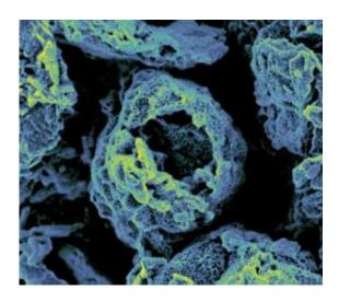
Using a new approach, the team built a graphene membrane for use in lithium-air batteries, which could, one day, replace conventional batteries in electric vehicles. Resembling coral, this porous graphene material could replace the traditional smooth graphene sheets in lithium-air batteries, which become clogged with tiny particles during use.
