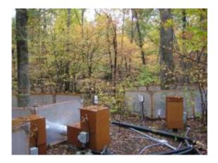
Five meter-wide, open-top chambers on the ground of the forest. Air is circulated through the tubes and raised by blowers into the chambers.
