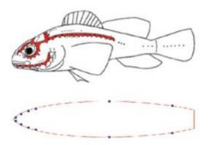
'Lateral lines; in fish contain hundreds of tiny pressure and velocity sensors that enable them to navigate through currents and eddies as efficiently as possible. To mimic that ability, MIT researchers have developed inexpensive, sensitive MEMS-based pressure sensors and mounted them on a small experimental vessel in a pattern that replicates the distribution of the lateral lines.
