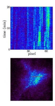
(Top) A "waterfall" plot showing the evolution of a cross section of a speckle pattern near the (00.2) HCP peak of cobalt during its martensitic phase transformation. Pattern discontinuities, such as the one at approximately 8 minutes, indicate the occurrence of avalanches. (Bottom) A single frame of the complete speckle pattern. The cross section used for the waterfall plot is indicated by the red line, which has a length of 5x10-3 inverse angstroms.
