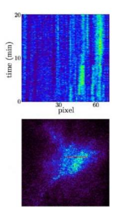
(Top) A "waterfall" plot showing the evolution of a cross section of a speckle pattern near the (00.2) HCP peak of cobalt during its martensitic phase transformation. Pattern discontinuities, such as the one at approximately 8 minutes, indicate the occurrence of avalanches. (Bottom) A single frame of the complete speckle pattern. The cross section used for the waterfall plot is indicated by the red line, which has a length of 5x10-3 inverse angstroms.
