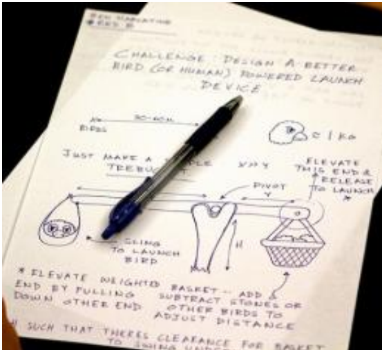
The design for one team's launch device for the MIT Angry Birds competition. Credit: MIT Course 2.009
