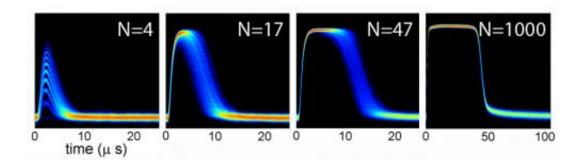
This series of data read-outs shows how the TES relaxation time increases with photon number. For N=4 photons, the TES returns from the elevated-resistance state to the edge of the transition region in less than 10  $\mu$ s. At N=47 photons, it takes around 15  $\mu$ s. And when the count is 1000, the relaxation time is approximately 50  $\mu$ s.
