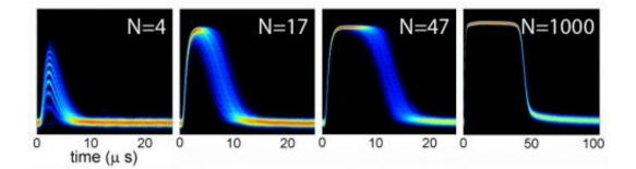
This series of data read-outs shows how the TES relaxation time increases with photon number. For N=4 photons, the TES returns from the elevated-resistance state to the edge of the transition region in less than 10  $\mu$ s. At N=47 photons, it takes around 15  $\mu$ s. And when the count is 1000, the relaxation time is approximately 50  $\mu$ s.
