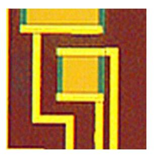
At the center of this micrograph, the TES is the orange-and-green square between two bright gold electrodes. Its dimensions are 25 X 25  $\mu$ m. Credit: NIST/PML
