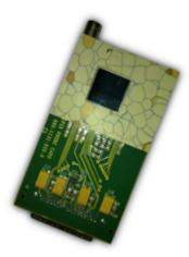
The Medipix device, shown here with protective plastic around the ultrasensitive chip.
