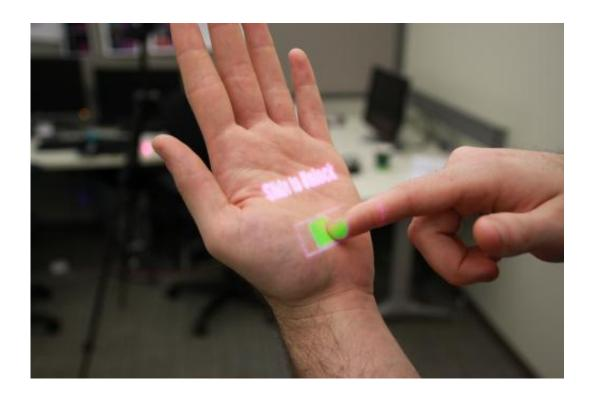
(PhysOrg.com) -- OmniTouch, a wearable projection system developed by researchers at Microsoft Research and Carnegie Mellon University, enables users to turn pads of paper, walls or even their own hands, arms and legs into graphical, interactive surfaces.
