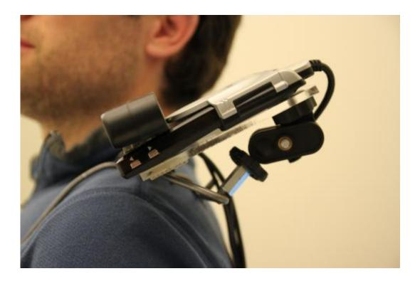
The OmniTouch device includes a short-range depth camera and laser pico-projector and is mounted on a user's shoulder. But Harrison said the device ultimately could be the size of a deck of cards, or even a matchbox, so that it could fit in a pocket, be easily wearable, or be integrated into future handheld devices.
