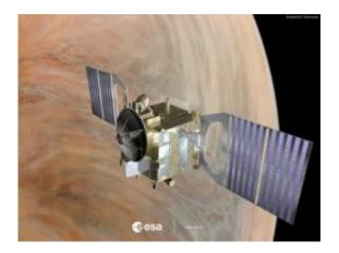
Venus Express has two solar cell panels per wing comprising alternating rows of standard triple junction solar cells as well as highly reflective mirrors to reduce the operating temperatures. There is twice as much sunlight in Venus's orbit as there is in Earth's orbit, plus additional thermal input from the Venusian surface and atmosphere - 75% of sunlight being reflected up from it. In certain cases, this results in Venus Express receiving an equivalent of the thermal input from 3.5 Suns.
