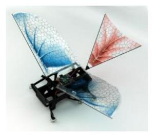
A dynamic hexapedal robot with flapping wings (DASH+Wings) for flapping wings configuration. Image: University of California at Berkeley
