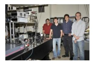
Drs. Joseph Melinger, Paul Cunningham, Joseph Tischler and Matthew Lumb next to a two-color femtosecond laser pump-probe apparatus used to measure the efficiency of multiple exciton generation in PbSe semiconductor nanocrystals and nanorods.
