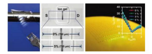
(Left) Graphene-based transistor patterned on a PDMS substrate. (Center) Microscope images of the transistor undergoing stretching up to 5%. (Right) The transistor patterned on a balloon. Image credit: Lee, et al. ©2011 American Chemical Society
