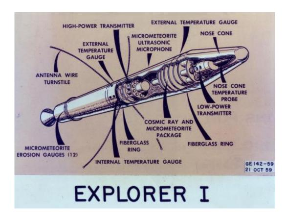
An exploded view of the first successful U.S. satellite launched in 1958, Explorer I. Credit: NASA/Marshall Space Flight Center Collection
