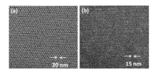
Scanning electron microscopy images of magnetic bits at densities of (a) 1.9 Terabit/in2 and (b) 3.3 Terabit/in2 formed after depositing Co/Pd multilayers onto resist structures.
