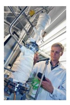
A researcher checks whether the soot particle filter is freed from soot even at exhaust temperatures of 140 degrees Celsius. (© Fraunhofer ISE)
