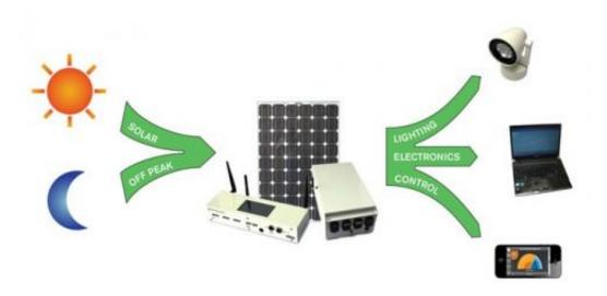
In Moixa Technology's Smart DC network, solar panels and off-peak electricity from the grid are managed by a hub, which provides power for computers and other low-power DC devices without the need for an AC/DC adaptor. Image credit: Moixa Technology
