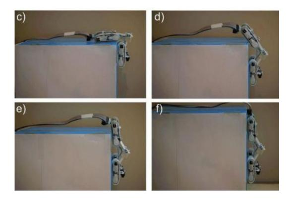
A tank-like robot that can scale vertical walls and crawl over ledges without using suction cups, glue or other liquid bonds to adhere to the surface. The 240-gramme (6.9-ounce) beast has tracks that are covered with dry microfibres modelled on the toe hairs of the gecko, which can famously zip up windows and along walls almost without effort.
