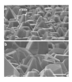
SEM images of GaN polycrystals grown on templates with LT-GaN/Ti/glass (a) and LT-GaN/glass (b). Scale bars are 2um. Image: *Nature Photonics*, doi:10.1038/nphoton.2011.253
