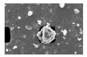
This is a close up of a single dust particle on the sensor. Credit: Images courtesy of Ohio State University.
