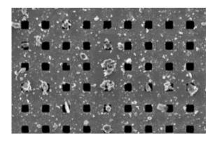
This is a sample of dust particles on the sensor surface. Credit: Images courtesy of Ohio State University.
