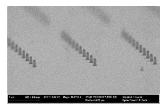
SEM image of the diamond nanoposts. Each one is approximately 100nm wide and 200nm tall. A nanometer is a billionth of a meter. Image courtesy of Jennifer Choy.
