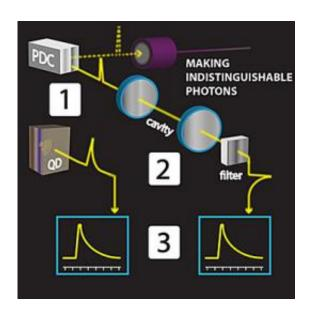
[1] A single photon is produced by a quantum dot (QD). Simultaneously, a pair of photons is produced by a parametric down-conversion crystal (PDC). [2] One of the PDC photons—which has different characteristics than the QD photon—is routed into a cavity and filter, [3] rendering this PDC photon and the QD photon nearly identical. Credit: Suplee, NIST
