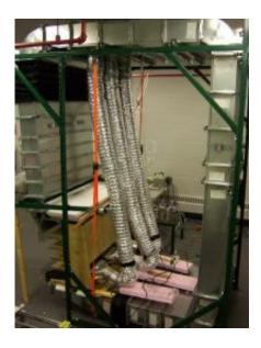
The experimental setup includes a half-scale display case shown in the lower left. Movable ducts adjust the settings for the air curtain that shoots across the opening. Credit: Image courtesy of Mazyar Amin
