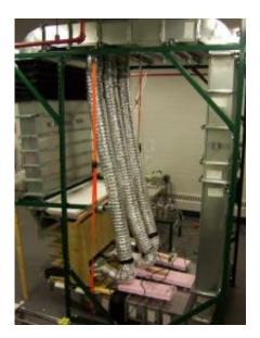
The experimental setup includes a half-scale display case shown in the lower left. Movable ducts adjust the settings for the air curtain that shoots across the opening. Credit: Image courtesy of Mazyar Amin
