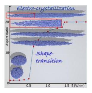
Electrocrystallization. Shape transitions and predicted electrocrystallization of a 10 nanometer formamide nano-droplet, obtained through molecular dynamics simulations. The vertical axis shows the aspect ratio between the long and short axes of the droplet.
