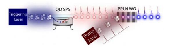
The color and shape of single photons produced by a quantum dot single photon source (QD SPS) are changed by combining them with a strong, pulsed pump laser in a nonlinear crystal (PPLN WG).
