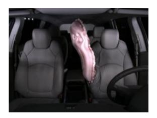
General Motors will introduce the industry's first front center air bag to help protect drivers and front passengers in far-side impact crashes where the affected occupant is on the opposite, non-struck side of the vehicle.
