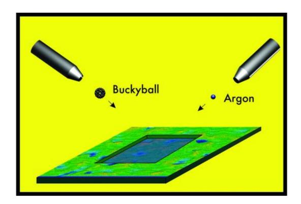
The rectangular depression is the result of multiple bombardments of the surface with buckyballs and argon during a depth-profiling procedure. Credit: Zbigniew Postawa, Jagiellonian University, Poland
