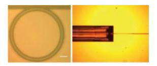
Researchers have created a tiny "microring resonator," at left, small enough to fit on a computer chip. The device converts continuous laser light into numerous ultrashort pulses, a technology that might have applications in more advanced sensors, communications systems and laboratory instruments. At right is a grooved structure that holds an optical fiber leading into the device. Credit: Birck Nanotechnology Center, Purdue University
