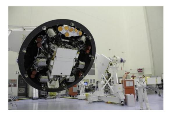
At the Payload Hazardous Servicing Facility at NASA's Kennedy Space Center in Florida, the "back shell powered descent vehicle" configuration of NASA's Mars Science Laboratory is being rotated for final closeout actions. Image Credit: NASA/JPL-Caltech
