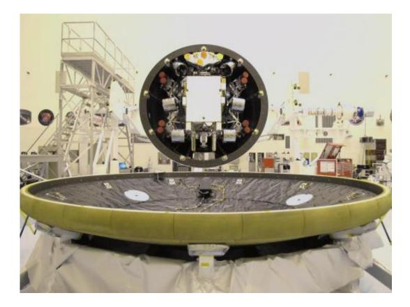
At the Payload Hazardous Servicing Facility at NASA's Kennedy Space Center in Florida, the "back shell powered descent vehicle" configuration, containing NASA's Mars Science Laboratory rover, Curiosity, is being rotated for final closeout actions. The flat, circular object in the foreground of the image is the spacecraft's heat shield. Image Credit: NASA/JPL-Caltech
