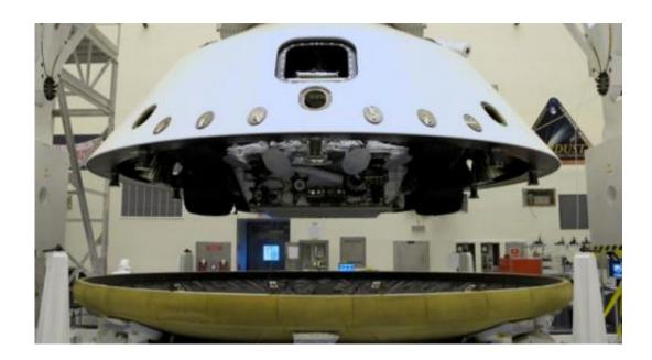
At the Payload Hazardous Servicing Facility at NASA's Kennedy Space Center in Florida, the "back shell powered descent vehicle" configuration, containing NASA's Mars Science Laboratory rover, Curiosity, is being placed on the spacecraft's heat shield. Image Credit: NASA/JPL-Caltech
