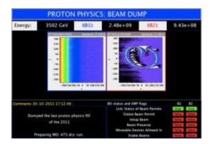
LHC control screen displaying the dump of the last beams for the LHC's 2011 proton run. The image on the right shows the cross section of the beam just before it was stopped. Credit: CERN
