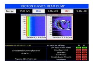
LHC control screen displaying the dump of the last beams for the LHC's 2011 proton run. The image on the right shows the cross section of the beam just before it was stopped. Credit: CERN
