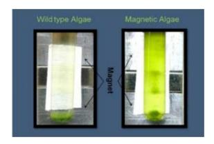
The photos show wild type algae and magnetic algae placed in a test tube next to a permanent magnet. The wild type (left) settles to the bottom of the tube under the influence of gravity. The genetically transformed algae (right) stick to the wall due to magnetic attractions.
