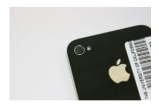
This is an iPhone microscope. It consists of a 1-millimeter-diameter ball lens embedded in a rubber sheet and taped over the smartphone's camera. Credit: Z. J. Smith, K. Chu, A. R. Espenson, M. Rahimzadeh, A. Gryshuk, M. Molinaro, D. M. Dwyre, S. Lane, D. Matthews, S. Wachsmann-Hogiu.
