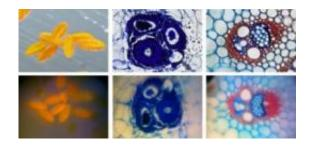
These are stained samples of pollen (left images) and plant stems (right two images). Top row: commercial microscope. Bottom row: cell phone microscope. Credit: Z. J. Smith, K. Chu, A. R. Espenson, M. Rahimzadeh, A. Gryshuk, M.
