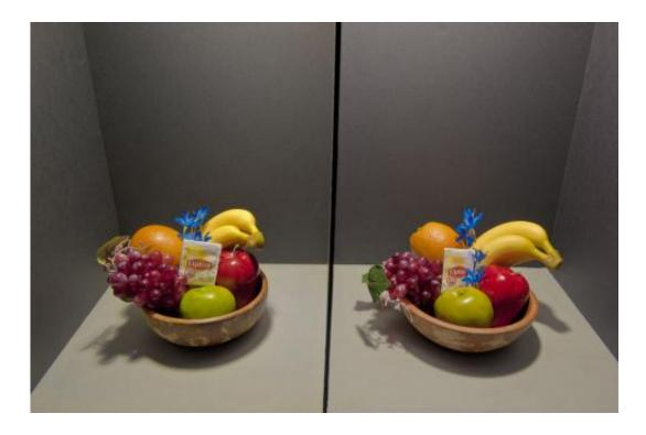
In the test setup, similar bowls of fruit were placed in a lightbox with a divider in the middle. In this photo, the bowl on one side was illuminated by a diode laser light and the other was lit by a standard incandescent bulb. The aesthetic quality of diode laser lighting (left bowl) compares favorably with standard incandescent lighting (right). (Photo by Randy Montoya).
