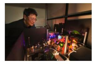
Sandia researcher Jeff Tsao examines the set-up used to test diode lasers as an alternative to LED lighting. Skeptics felt laser light would be too harsh to be acceptable. Research by Tsao and colleagues suggests the skeptics were wrong. (Photo by Randy Montoya).
