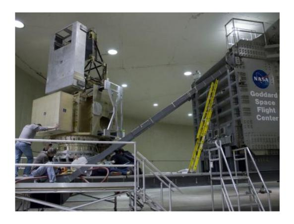
The GPM satellite, under construction, is fitted to the bed of the High Capacity Centrifuge for spin testing. Credit: NASA/Goddard/Rebecca Roth
