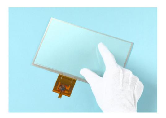
(PhysOrg.com) -- A new screen has been designed that can work with gloved hands, and it comes from Japan-based SMK. The target application will be car-navigation systems which drivers can operate while wearing gloves. The new screen is described as having a sensor panel structure that is noise-resistant. The design allows for a signal clear enough to be detected at high sensitivities.
