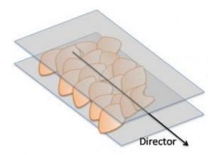
Graphene oxide flakes in a solution align themselves with a director, a dimensionless vector that represents the preferred orientation of particles in a liquid crystal. Credit: Rice University/University of Colorado at Boulder
