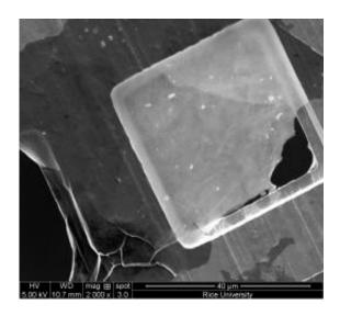
A single flake of graphene oxide roughly 40 microns wide, seen under an electron microscope, sits atop a copper support. Such "giant" flakes form into a gel-like liquid crystal in solution. Credit: Rice University/University of Colorado at Boulder
