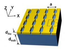
The proposed light-funneling structure consists of an alternating pattern of large and small slits engraved on a thin gold film on a substrate. The large slits increase the efficiency of the light funneling through the small slits, while the small slits provide tighter confinement for greater light enhancement. Image credit: G. Subramania, et al. ©2011 American Physical Society
