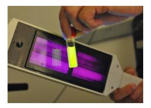
A liquid solution of a perylene dye, which emits a green fluorescent light is measured with a custom hand-held photodetector. Photo Credit: Courtesy of University of Utah Technology Venture Development
