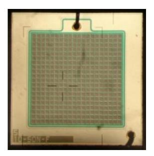
An MPPC detector consisting of an array of avalanche photodiodes. Credit: A\*STAR Research
