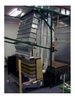
In the experimental setup, the air curtain exits out of the top of the case, flows down in front of the wooden shelving units, and then circulates through the ducts at the bottom of the case. Credit: Mazyar Amin
